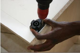
The last leg base is fitted inside the vertical and is set back by 20 mm. The side kickplate will then support the vertical of the cupboard.
